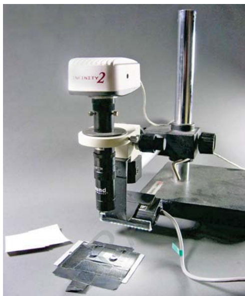
Figure 1. Microscope and light configuration for producing raking light photomicrographs.
